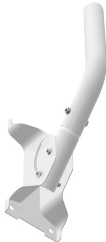
The Mimosa Advanced J-Mount accessory accommodates most under roof eave mounting applications. With an extra axis of rotation to align the C5 and keep it level to the horizon, the J-Mount provides three degrees of rotation for elevation, azimuth and pole twist adjustment for precise aiming.
